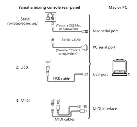
Note: Before you connect to serial or MIDI ports, turn off your Yamaha mixing console and computer.
