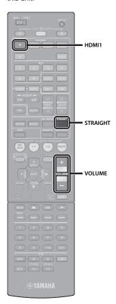
1 Press HDMI1 to select "HDMI1" as the input source.
