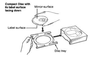
3. Line the disc tray up with the grooves in the magazine, and holding it by the knob, push the disc tray all the way in, until the tray clicks.
