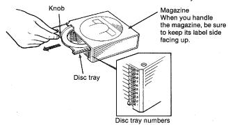
2. Draw the disc tray completely out of the magazine and place a Compact Disc on it with its label surface facing down.
