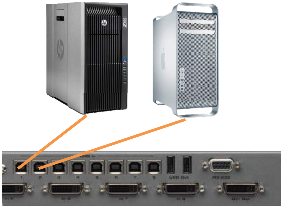
【Connection between KVM switch and computers】
