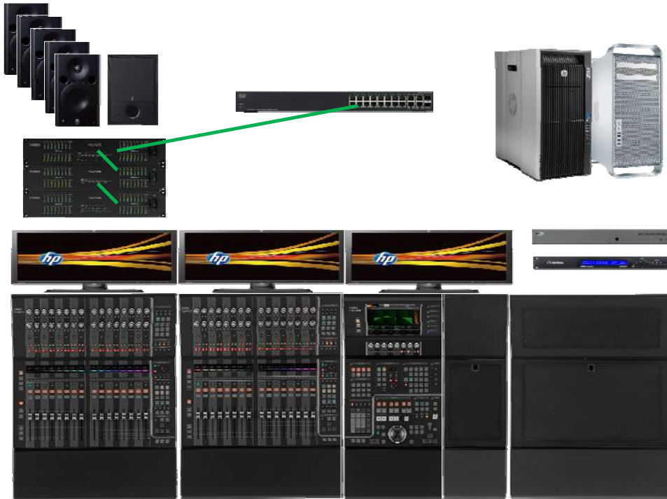
【Connection between switch and I/O(Daisy-chain Mode)】
