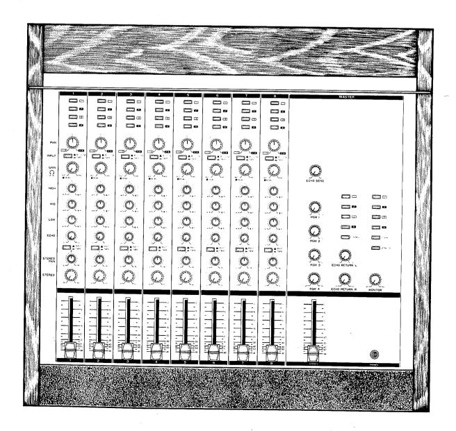
The RM804 is an 8-in/4-program-out mixer with many features including balanced mic/line inputs, an echo mixing buss, full monitoring capability and a SUB input for cascading a sub-mixer when more input channels are required. There are also continuously variable input gain controls for matching input sensitivity, 3-band equalization, and extensive VU metering for easy, accurate level control.
