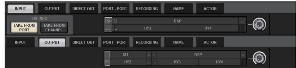
HY SLOT4 (HY SLOT3 on the CSD-R7) now supports input/output patches.
