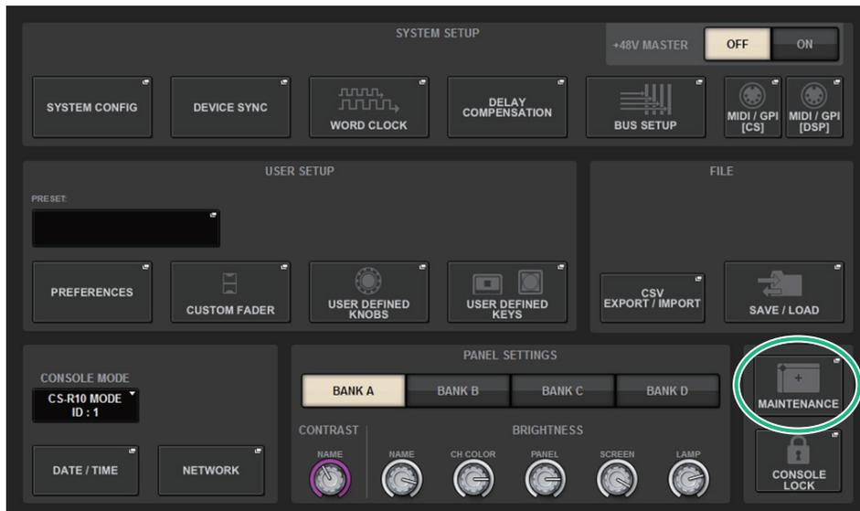
1. Press the SETUP button to access the SETUP screen.
