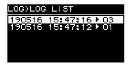
Turn the main knob to select an event, and then press the main knob to access the DETAIL VIEW screen. For details on the messages, refer to "Message list."
