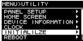
2. In the UTILITY screen, turn the main knob to select “INITIALIZE,” and press the main knob to confirm.
