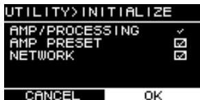
3. Turn the main knob to choose the type of settings that will be initialized (multiple selections are possible), and press the main knob to confirm.
