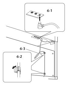
Insert the pedal cord securely until the metal part of the cord plug disappears from view.
