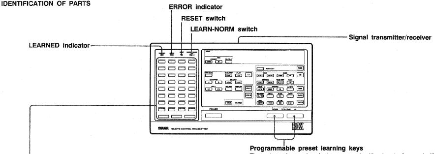
These keys can be used to "learn" (program) signals from other remote-control transmitters.
