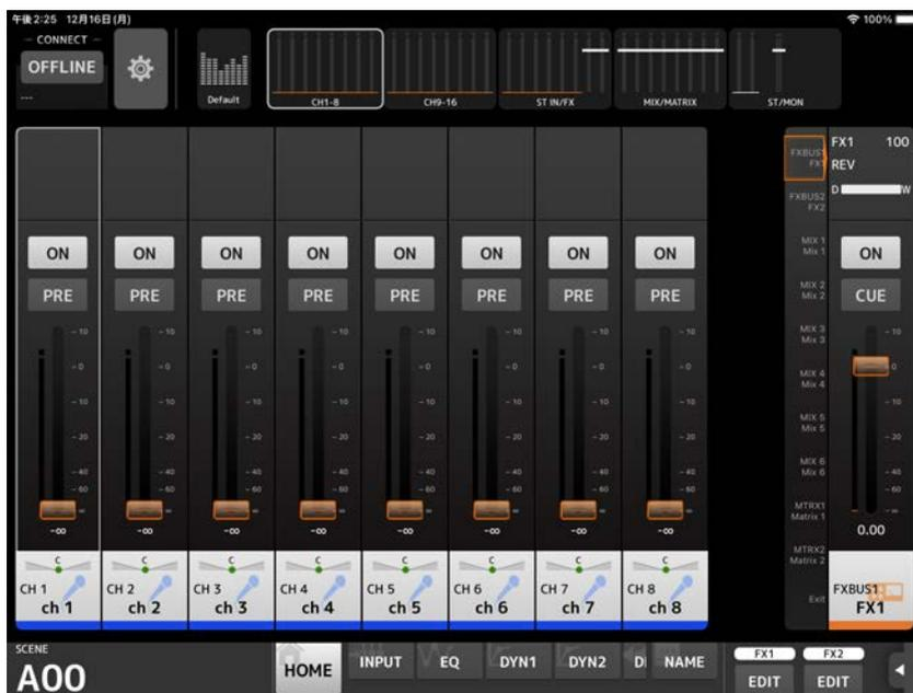
In SENDS ON FADER mode, the details area changes to display SENDS ON FADER information.
