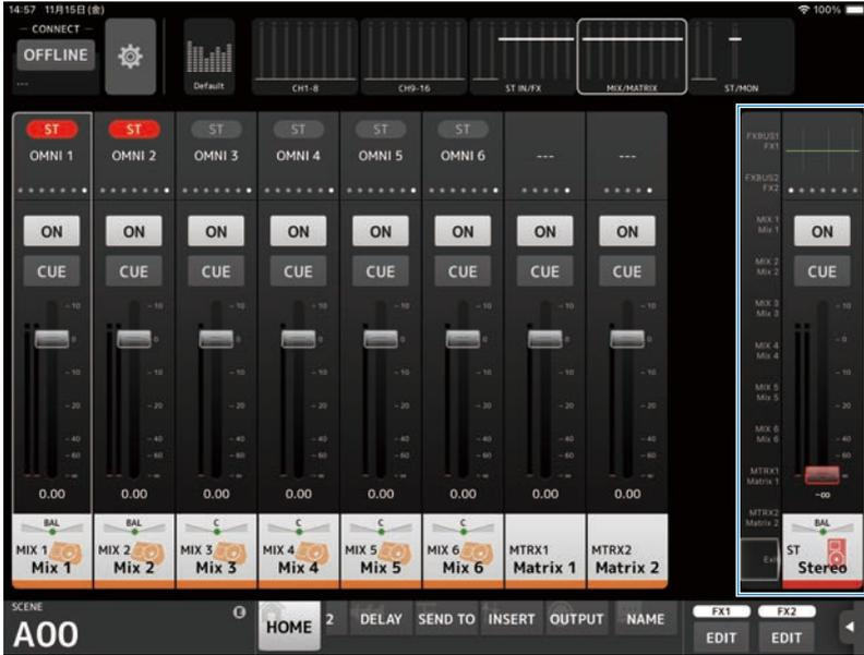
You can switch to the SENDS ON FADER mode by tapping the channel number on the left side of a strip. The selected channel is then highlighted in the channel's color. Tapping EXIT at the very bottom, or the selected channel number, restores the regular mode.
