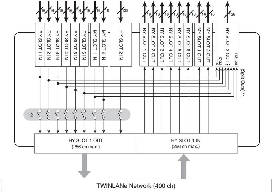
\*1) In mode 1, all input signals (total 128 channels) of the RY slots and MY slots are always split for output to the HY SLOT 2 output. The signal is output immediately after gain compensation.
