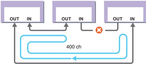
Even if a cable is severed at one point, the signal will be re-routed automatically and communication will continue without interruption.
