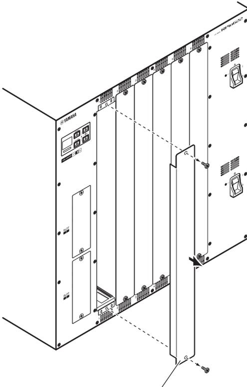
**3** **Align both edges of the card with the guide rails inside the slot, and then insert the card into the slot.**
