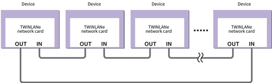
If a cable in the network breaks down for some reason, the signal will be automatically re-routed and audio will flow without interruption. Even if a device in the network malfunctions, other working devices will be able to continue communicating.
