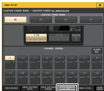
Finestra USER SETUP (pagina CUSTOM FADER BANK/ MASTER FADER )
