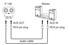
When these are connected (with RCA pin plug; LEVEL FIXED), the sound is output to the external device at a fixed level, regardless of the [MASTER VOLUME] slider setting.
