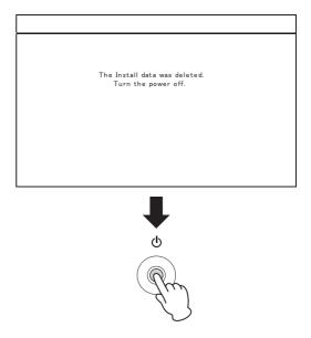
Turn off the STAGEA and disconnect the USB flash drive.
