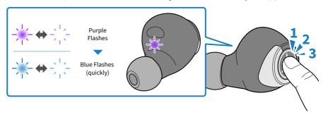
If the indicator displays as shown below after several seconds, initialization was successful and the earphone enters standby mode for pairing with a Bluetooth device. If the indicators are not displaying as shown, try initializing once more from step 1.
