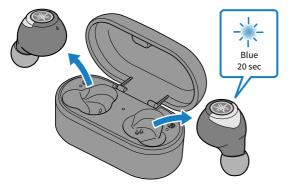
If they do not automatically connect, the earphones will enter connection/registration (pairing) standby mode. Initiate the connection to the earphones from your Bluetooth device.
