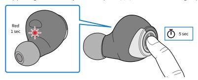
2 Hold down the function key on earphone (L) for about 10 seconds. and the indicator flashes as shown below.
